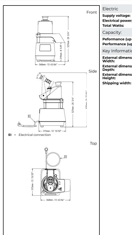
Electric Supply voltage: 115 V/1N ph/60 Hz Electrical power, max: 1kW **Total Watts:** 1kW Capacity: Peformance (up to) 330,6 lbs/cycle Performance (up to): 150 kg/Cycle Key Information: External dimensions, Width: 13 11/16" (348 mm) External dimensions, 12 3/8" (315 mm) Depth: External dimensions, 20 3/4" (527 mm) Height:
